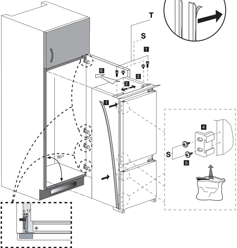
**Note:** Installation step for 2, screws for connecting top plastic part should not be screwed very hard, because of moving the plastic part easily left or right side.
