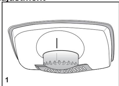
Operating temperatures are controlled by the thermostat knob (see diagram) located on the ceiling of fridge compartment. Settings may be made from 1 to 5, 5 being the coldest position.
